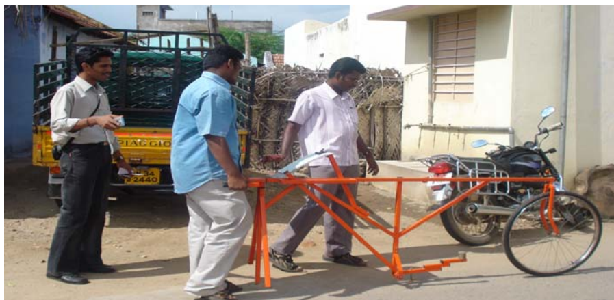
Photo: Testing of Roughness using MERLIN
